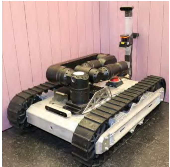
Fig. 1. Robot in expected final assembly configuration. The arm is folded back for storage and navigation.
