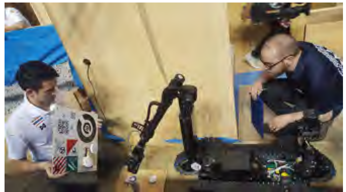
Fig. 6. Robot manipulator arm has a camera and a gripper at the end effector.
