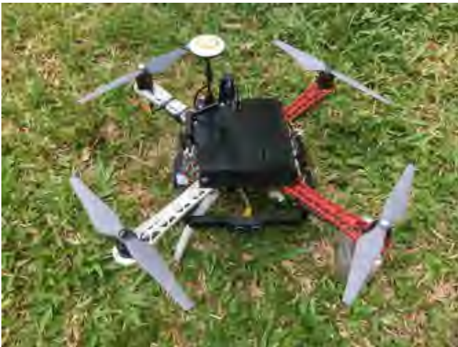
Fig. 4. Autonomous flying robot in outdoor mission, as quadrotor model.
