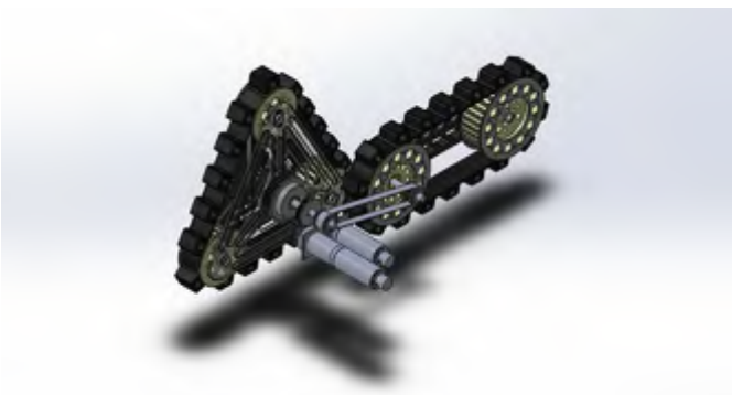
Fig. 4. Mechanical design of right side tracks
