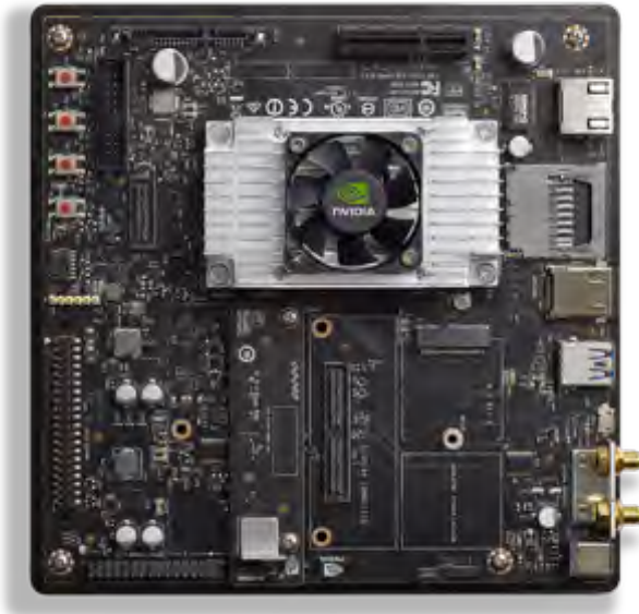
Fig. 2. NVIDIA Jetson TX2 Developer Kit
