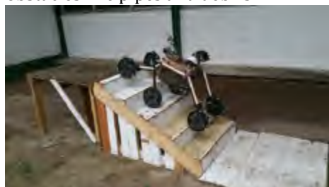
Figure 4: First test of the structure climbing stairs.
