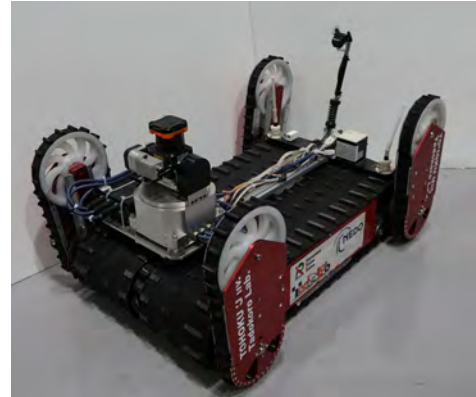
Fig. 1. Tracked vehicle “Quince”. We use this robot as a mobile base.
