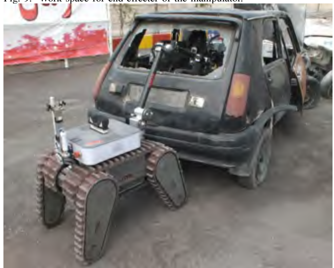
Fig. 10. Karo is inspecting inside a car using the 6-DOF manipulator.
