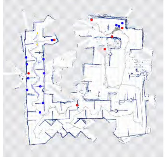
Fig. 14. Illustrates the generated merged map by MRL autonomous and tele-operative robots at the final mission of RoboCup 2015.
