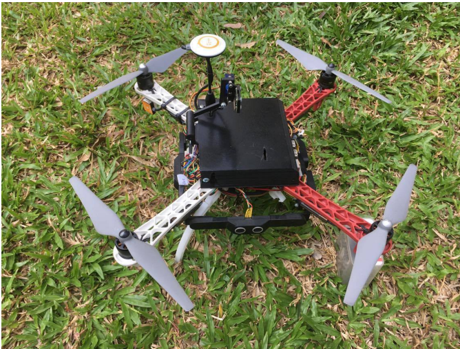
Fig. 3. Autonomous flying robot in outdoor mission, as quadrotor model.
