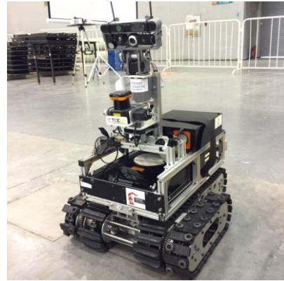
Fig. 2. The previous iteration of the autonomous robot of BART LAB Rescue Robotics team, AutoBot IV, this robot has a track-based locomotion system with sensors for the victim identification system, which uses image processing and heat imaging
