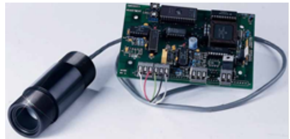
Fig.6.1 IR Sensor model OS65 used for body temperature measurement
