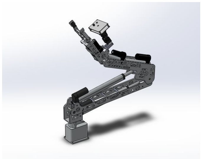
Fig. 8: Hurtash robot arm with 8 Degree Of Freedom (DOF)
