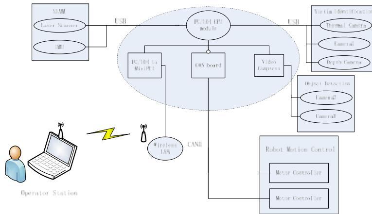
**Fig.4 Diagram of the autonomous robot control hardware structure**
