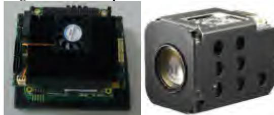
**Fig. 6 Embedded computer and camera on tele-operative robot**
