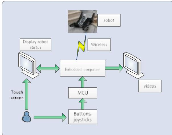
**Fig. 16 Hardware structure of control box**
