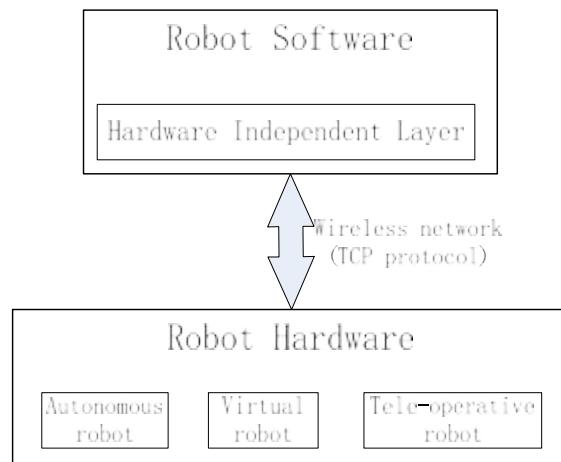
**Fig. 8 The control method of software**
