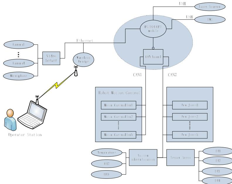
**Fig. 5** Diagram of the tele-operative robot control hardware structure
