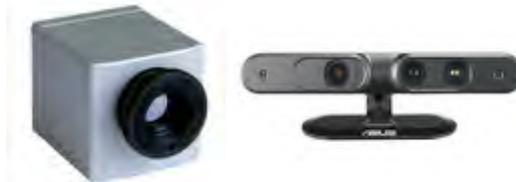
**Fig. 13 Thermal Camera & Depth Camera for Victim Identification**
