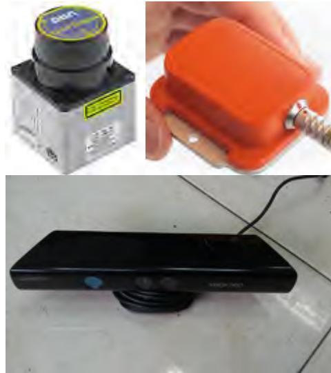
**Fig. 12 Scanning Laser Range Finder & IMU & Kinect**
