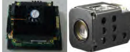
**Fig. 6** Embedded computer and camera on tele-operative robot
