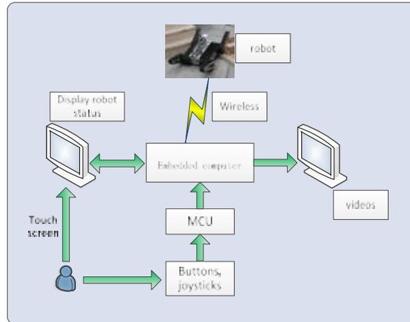
**Fig. 16 Hardware structure of control box**
