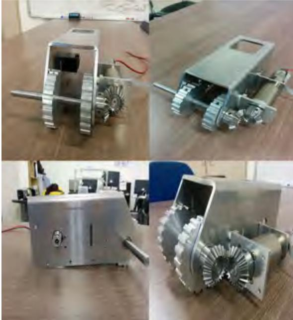
Fig. 3. Photo of robot's main driving part (one module)
