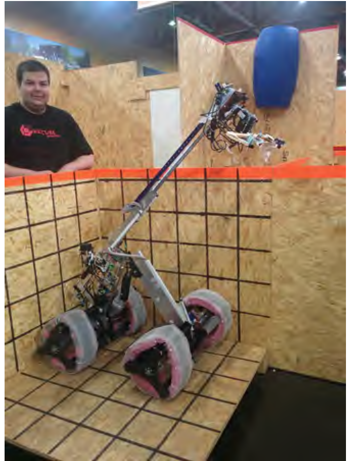
Fig. 9. The variable geometry with a linear neck mechanism
