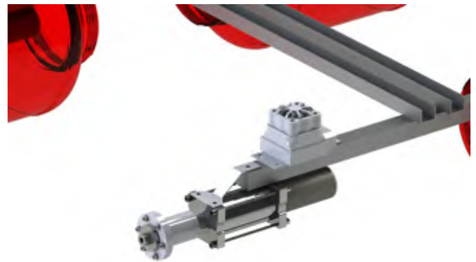
Fig. 5. The planned 2016 robot has a twisting body with an arm attached on one end
