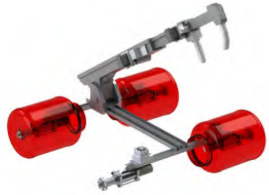
Fig. 5. The planned 2016 robot has a twisting body with an arm attached on one end
