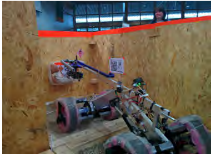
Fig. 3. Variable geometry allows the robot to navigate the sensors near this victim
