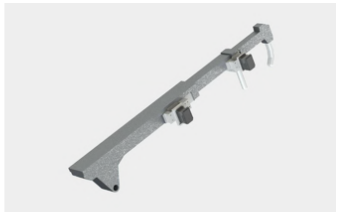
Fig. 10. The arm has linear actuators, with grippers attached
