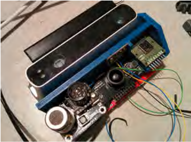
Fig. 11. Sensory head with thermal camera, RGB camera, depth camera and ultrasonic, CO 2 , inertial sensors
