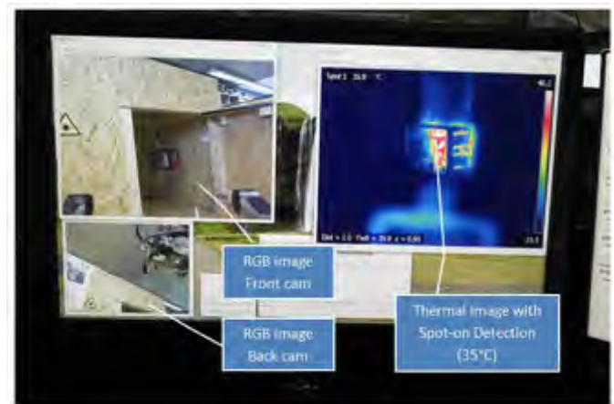
Fig. 9. View of RGB and thermal camera for victim detection
