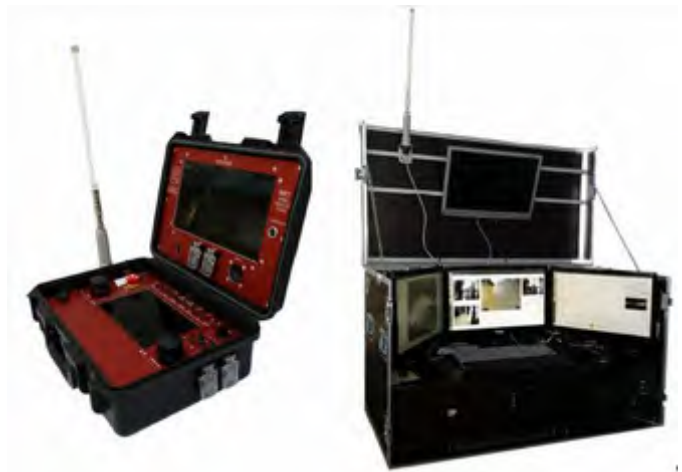
Fig. 8. RRT Remote Control Unit (RCU 2000 and RCU 3000)
