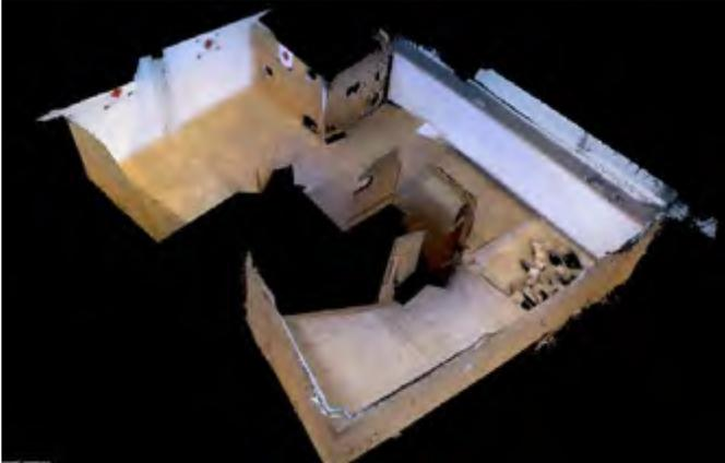
Fig. 13: Partial reconstruction of a RoboCup arena based on RGB-D data.
