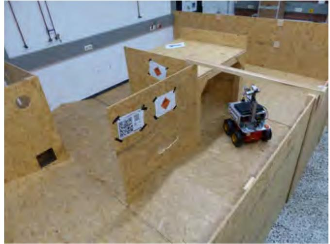
Fig. 16: Arena-like experimental setup with RoboCup elements including ramps, a stepfield and a tunnel.
