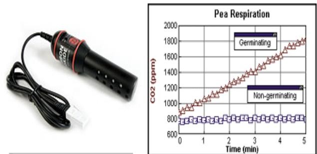
**Fig 6.2:** CO<sub>2</sub> sensor and response.
