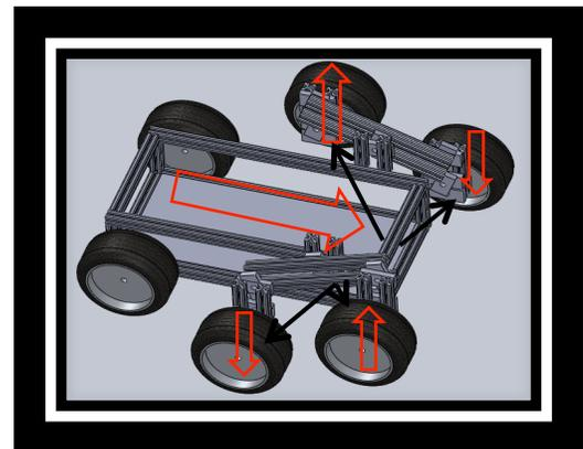
**Fig 7.2** Mechanic movement of structural mobile robot
