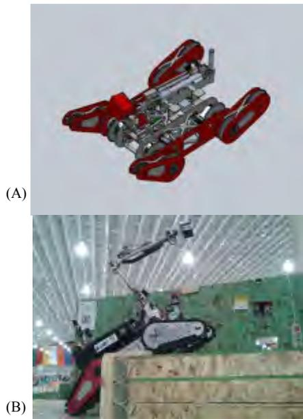
Fig. 3. (A) CAD of TeleOp V platform (B) TeleOp V in step field
