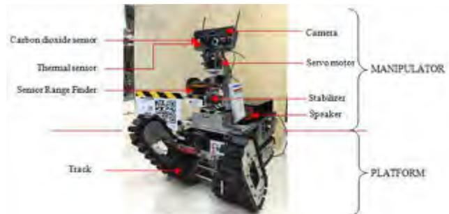
Fig. 6. Components of autonomous robot
