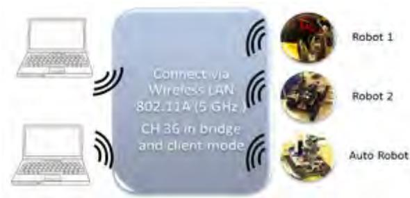
Fig.12. Diagram of the operator station
