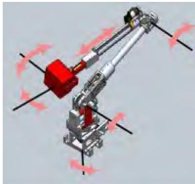
Fig. 4. CAD representation of the six degrees-of-freedom manipulator
