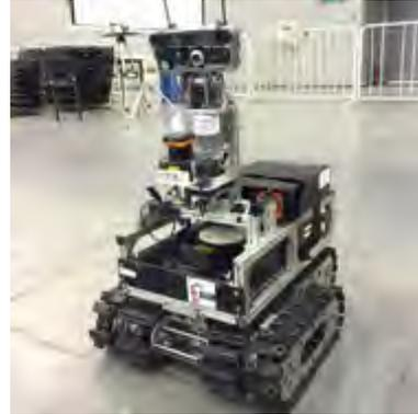
**Fig. 2.** Autonomous robot of BART LAB Rescue Robotics team, AutoBot IV. This robot has a track-based locomotion system with sensors for the victim identification system, which uses image processing and heat imaging technology.
