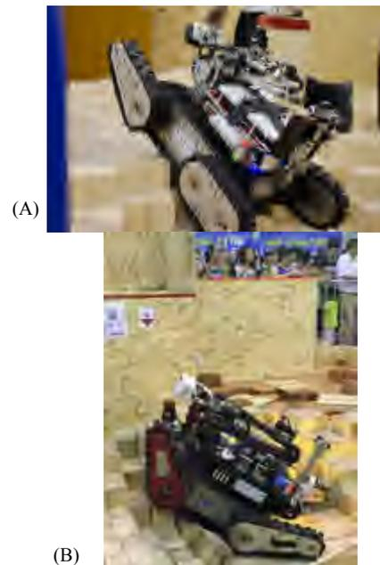
**Fig. 1.** TeleOp IV - our previous version (A) and TeleOpV (B) are the two tele-operative robots in BART LAB Rescue Robotics Team. Both robots employ track locomotion with four independent flippers, and are equipped with manipulator which is controlled using inverse-kinematic algorithm for their capabilities in search and retrieve victim information, similarly to robots in [1, 2].
