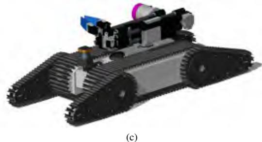
Fig. 1. Robot's of team AutonOHM: Georg (a) is used for autonomous driving and exploration. Robot Simon (b) can further be used for teleoperated driving. The new robot (c) will be capable of driving in rough terrain. Equipped with a manipulator it can inspect points of interest up to a height of 1.5 meters.
