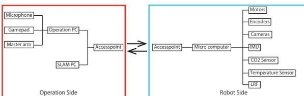
Fig. 14. system configuration
