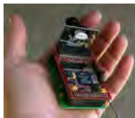
Fig. 3. RCM Blackfin Controller with OmniVision OV7725 camera.
