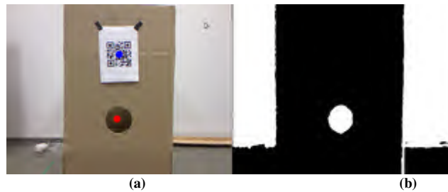
Fig. 7. Test Results of the developed system (a) QR-code is marked by blue dot while the hole is pointed out by red one and (b) black/white image obtained by medianization in the first step of hole detection
