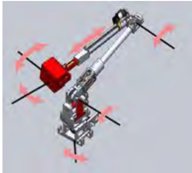
Figure 14: CAD representation of the six degrees-of-freedom manipulator
