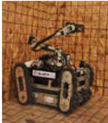
Figure 2: Autonomous robot of BART LAB Rescue Robotics team. This robot has a track-based locomotion system with sensors for the victim identification system, which uses image processing and heat imaging technology.
