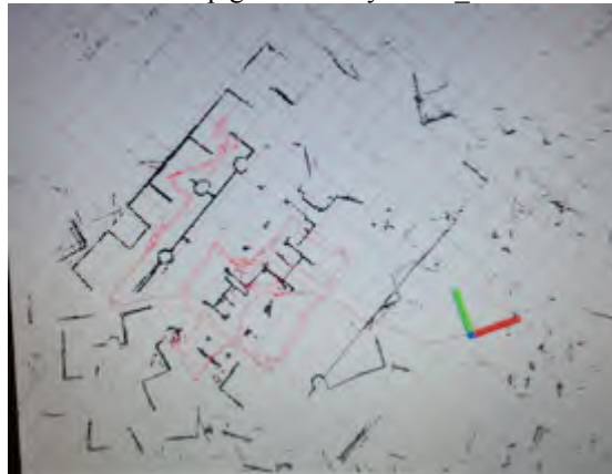
Figure 5: Automatic map generated by iRAP_ROBOT's software
