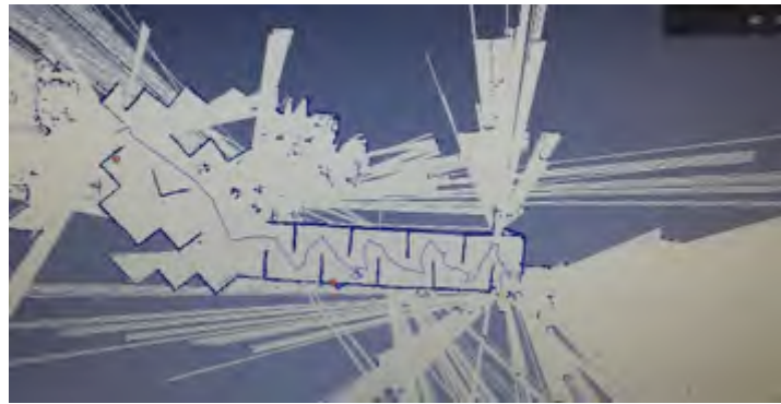
Figure 4: Automatic map generated by iRAP_ROBOT software
