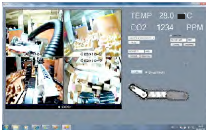
Figure 3: Operator console illustrated the real time quad videos And the information of robot's sensors.
