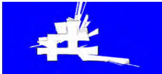
Fig. 5. Map of our test arena using ICP scan matching algorithm
