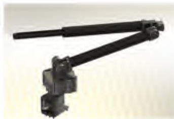
Fig. 9. New design of the 6 DOFs serial manipulator
