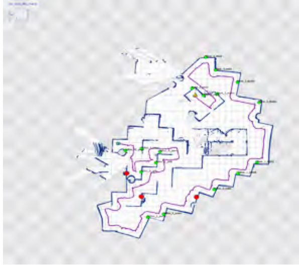
Fig. 15. Illustrates the generated map by MRL autonomous robot at the final mission of RoboCup 2012. The robot exploration started from middle of the arena and autonomously explored the arena and it was capable of finding 3 victims (red markers), and 17 QR codes (green markers).
