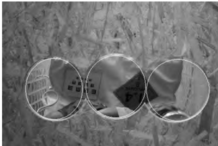
Fig. 11. Blob detector algorithm results on victim location in arena from a captured picture
