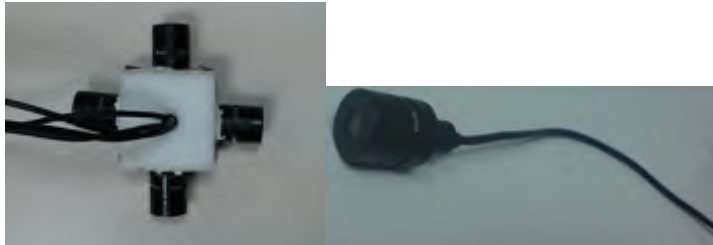
Fig. 13. The prototype coincident microphone array consisting of four JOGA EM1.3 cardioid electret microphones.
