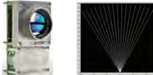
Fig. 9 The Leddar M16 sensor and its field of view
