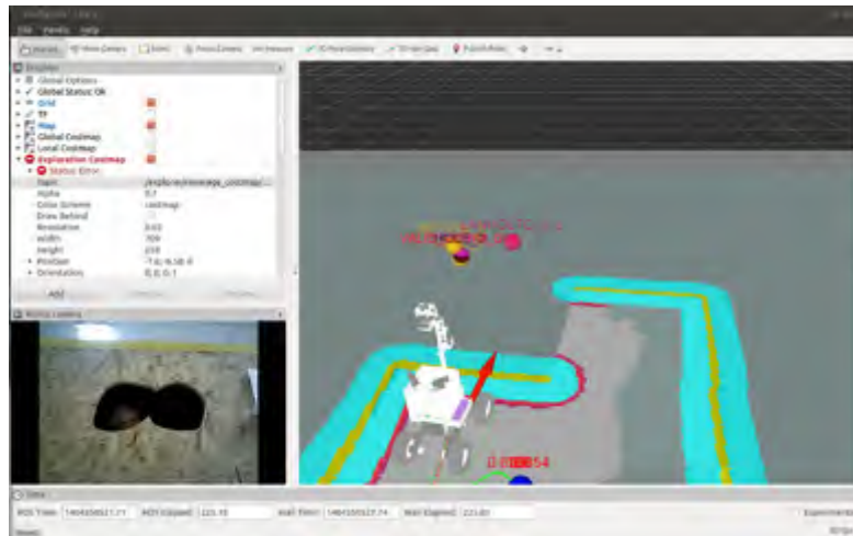
Fig. 3. Rviz GUI – Showing the perceived world model and a live stream from the robot's camera (bottom left).
