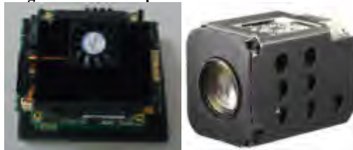
Fig. 6 Embedded computer and camera on tele-operative robot 4.3 UAV
