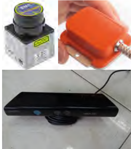
Fig. 12 Scanning Laser Range Finder & IMU & Kinect
