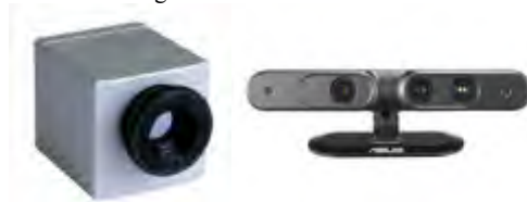
Fig. 13 Thermal Camera & Depth Camera for Victim Identification
