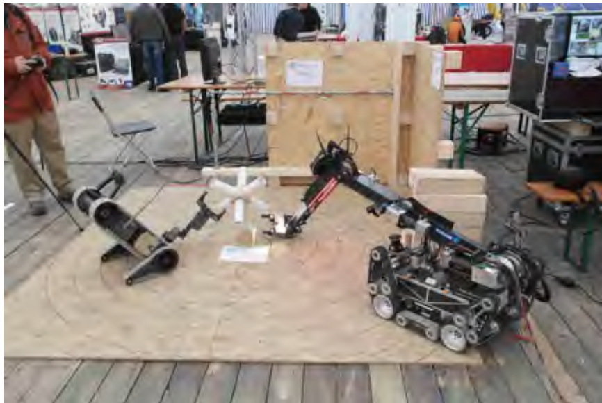
Figure 20: Pipe inspection with MARK and iRobot 310 SUGV
