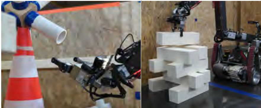
Figure 16: Pipe inspection and shoring task
